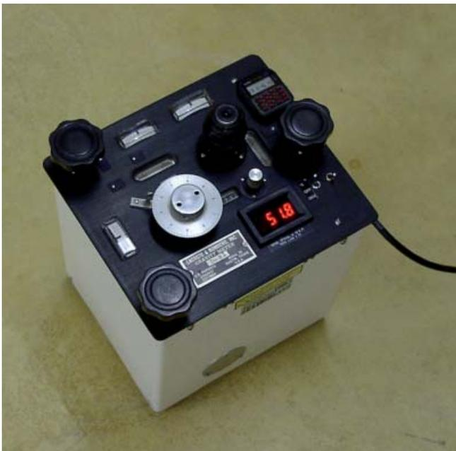
Abb. 5: Relativgravimeter LCR-D51, 1981 - 2010
